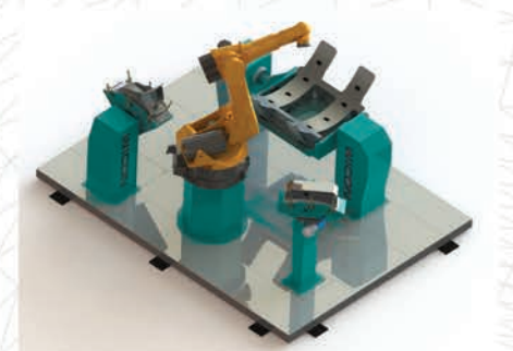
WFRS: Robotic Welding System with Fix- ture Equipment
